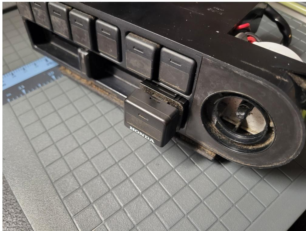
Push the delete in keeping in mind it only fits one way. The cut out/stepped section on the rear should face the blower knob, as shown here:
