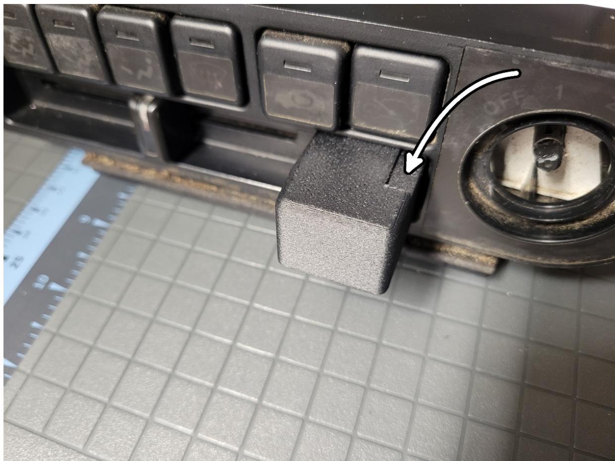
The delete has a tighter fit than the original A/C button did, this is intentional. You will need to push it firmly until it seats:
