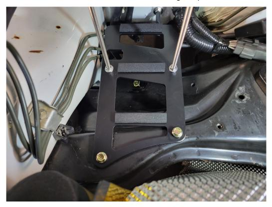
If you are using the K-swap heat shield install it now using the same front bolts:
