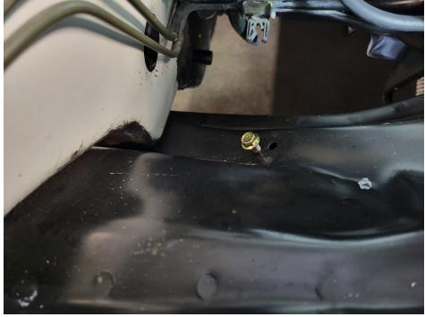
The battery tray rear mount has an open slot. Slide this under the bolt head when you place the tray onto the subframe:
