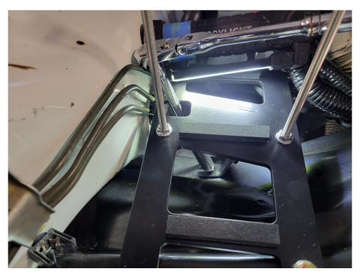
Place the battery on the tray and then the top tie down onto the battery. Center the battery so that the "restart" button is centered in the tie down:
