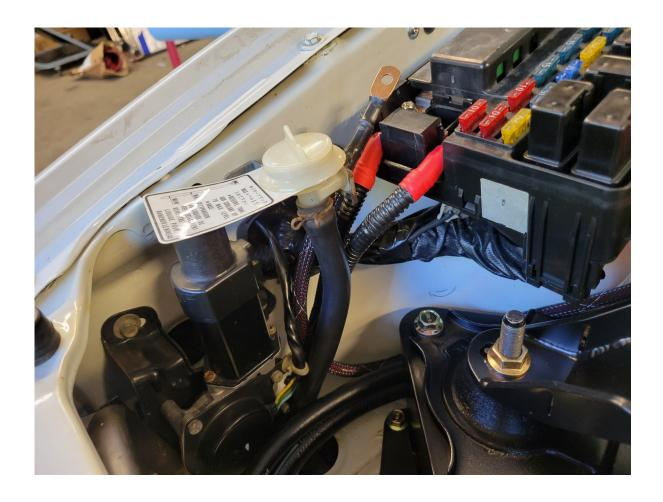
Remove the left fuse box cable bolt.
