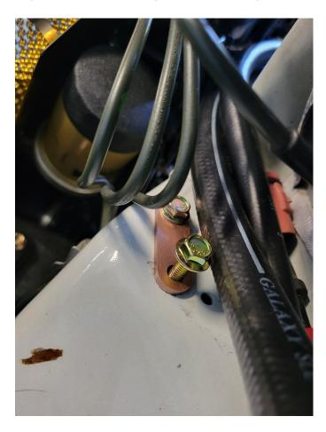
Route the cable like this but DO NOT connect it to the battery yet!:
