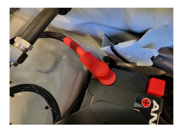
Route it along the side of the bay, keeping it tucked behind the brake and other lines. It will run down near the headlight motor then up to the fuse box:
