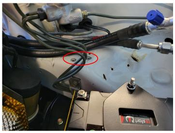
Before installing the spreader use a razor and carefully scrape away all the paint and primer around the holes.
