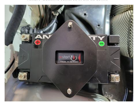
Finally, add the nylon locking nuts. Tighten each a little at a time and keep testing how secure the battery is. There are foam blocks on the tray and tie down that will squish as you tighten. Tighten until you are not able to shift the battery position by grabbing and tugging on it.
