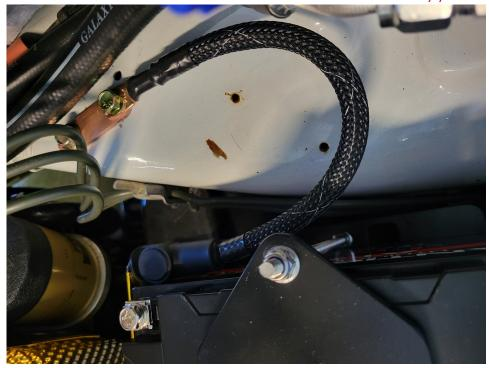
Install the positive cable onto the battery using the hardware supplied with the battery:
