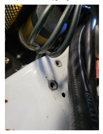
Use some dielectric grease between the chassis and ground spreader. I use a small paint brush to apply it. This grease will stop corrosion. It's also great to use on any other connections to stop corrosion. The grease can be messy on exposed surfaces. In that case I like to bush on some ACF-50:
