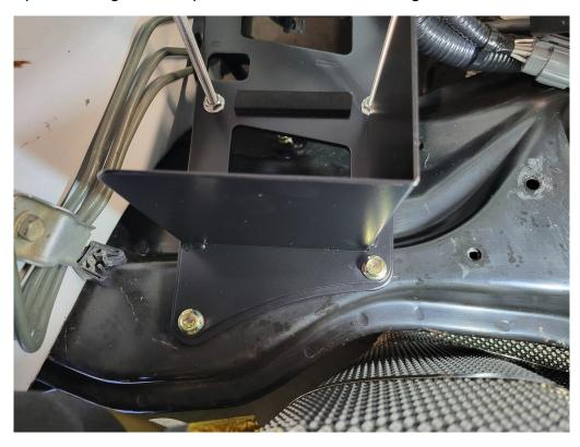
Tighten the rear 10mm bolt using an extension through the access hole in the tray. Then tighten the front bolts:
