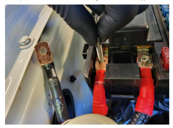
If you ordered the new starter cable also install it on this same stud (with the other end going to the starter). For proper fit put the battery and starter cable end with the ring terminal "hump" facing away from each other:
