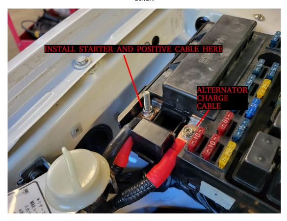
The live stud is intended as a convenient place to attach a battery tender or jump cable lead. Attaching leads directly to the battery is hard due to their size and location. Make sure you use the correct type of charger or tender for the ATX20-RS!
