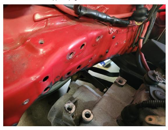
Install 4 adapter bolts finger tight only. Fully tighten the Allen flat head bolts first, then the last two:
