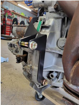
To install the timing side bracket start by removing the crank pulley and the lower timing cover. Next remove the factory mount bracket from the block, you should be at this point:
