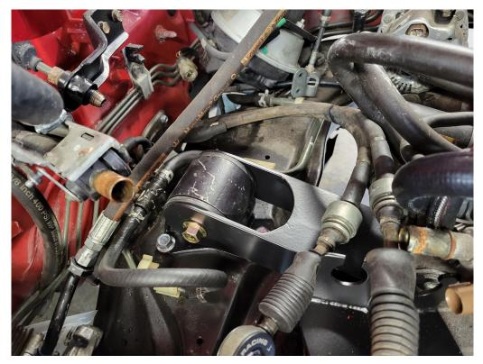
Install the transmission bracket onto the transmission and then install the 3g Prelude manual mount:
