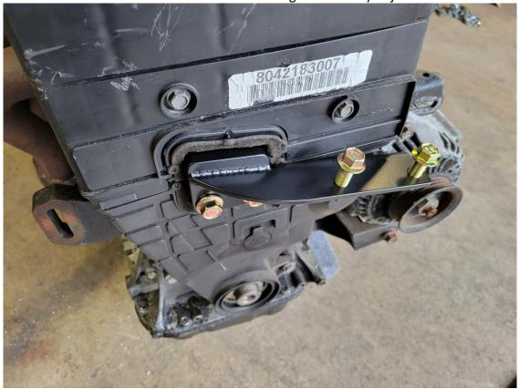
Leave the crank pulley and transmission mount bracket off until the motor is installed in the bay.
