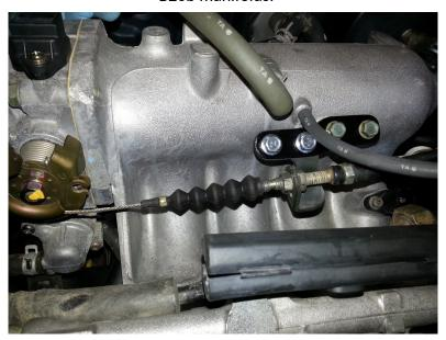
Here is what someone has done for their B18C swap with a GSR manifold. He welded the Prelude throttle bracket onto the GSR bracket. The throttle cable is just long enough:
