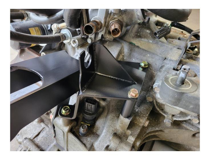
Install the front mount bracket onto the motor. Because B-series motors don't use a front mount this bracket bolts onto the engine using 3 of the transmission bell housing bolts. There are 2 different front swap bracket styles, one that mates to the OE Prelude mount and one that mates to the Prelude Engineering traction bar:
