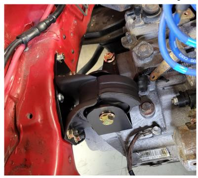
For the timing side install a B20a style mount and chassis side bracket. You can not use a B21 mount and chassis bracket:
