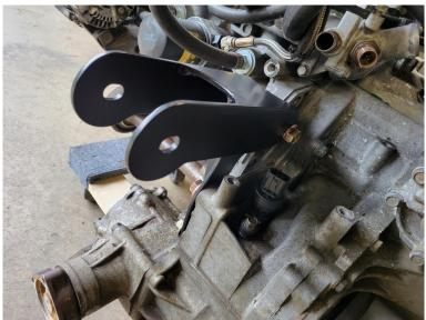
After installing the rear braket install the new shifter cable bracket:
