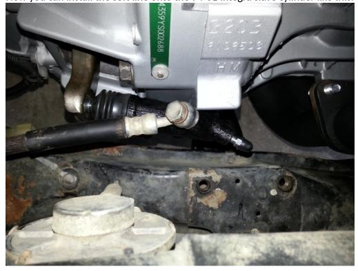
There is tight clearance between the slave cylinder and front mount bracket so you may need to install the soft line first, then bolt the slave cylinder onto the transmission.
