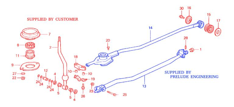
Your B-series swap mounts came with a shifter adapter plate, plus the bolts and nuts needed for it. Install the plate like shown (finger tight only), with the longer bolts hanging down:
