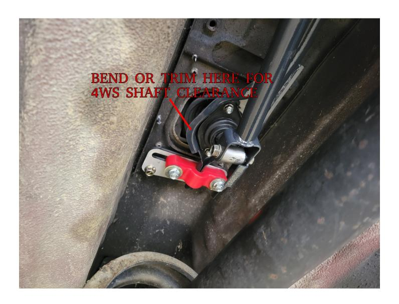
NOTE: If you are missing the metal support for the rear shifter bushing then you should at least use some large fender washers to support the bushing (we do recommend using the OE support if possible). The metal sleeves that fit inside the bushing holes are also required:
