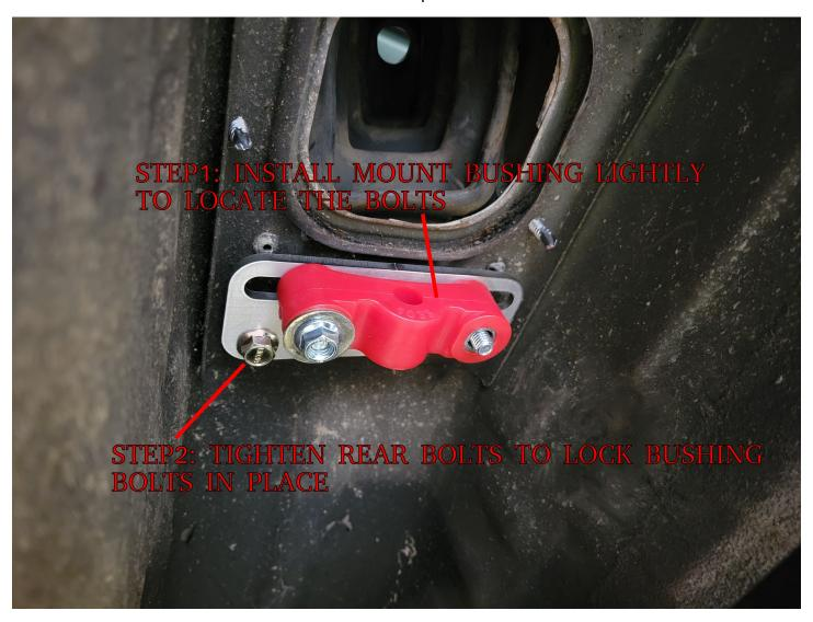
You will notice the adapter plate has slots. This allows you to adjust the position of the shifter to either side. I suggest starting in the middle position and if needed adjust later after everything is installed.
