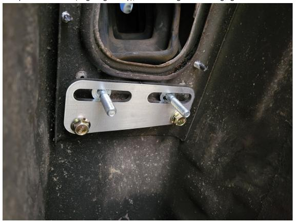
Briefly install the rear mount bushing to locate the long bolts then tighten the rear bolts. This will lock the long bolts into place:
