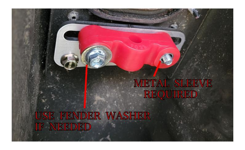
**Final step:** The adapter plates holes were never meant to support weight from below so you must install some nuts on the bolt threads sticking into the interior, do not skid this step:
