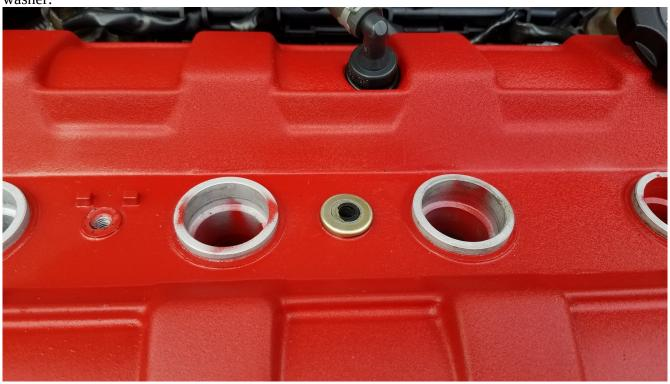
Place the supplied o-rings around the spark plug tubes. These stop water ingress from below the plate:
