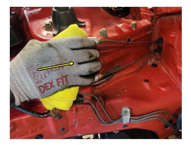
Push the valve back until its black mounting bracket matches up with the bend in the shock tower sheet metal like shown here:
