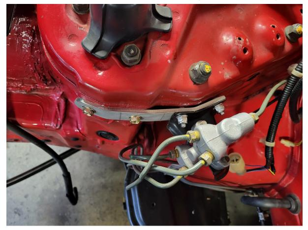
Tweak the shape of the brake lines on the front of the proportioning valve so that they don't touch each other or the chassis.
