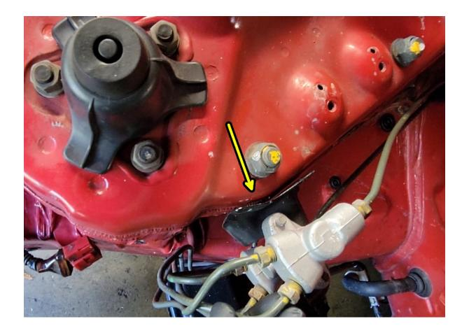
Install the relocation bracket on the proportioning valve bracket using the low-profile Allen bolts and nylon locking nuts like this:
