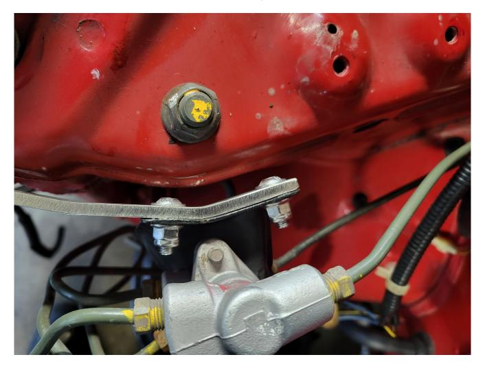
The front bracket holes probably won't line up perfectly at this point. Just bend the proportioning valve as needed to get them lined up.
