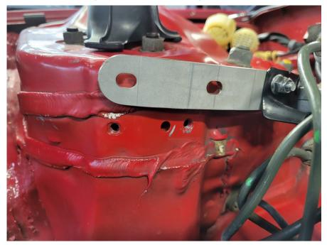
After that install the bracket bolts to secure everything to the shock tower again:
