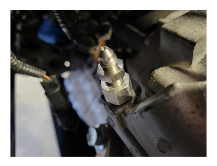
Install the 3AN soft line onto the new fittings:
