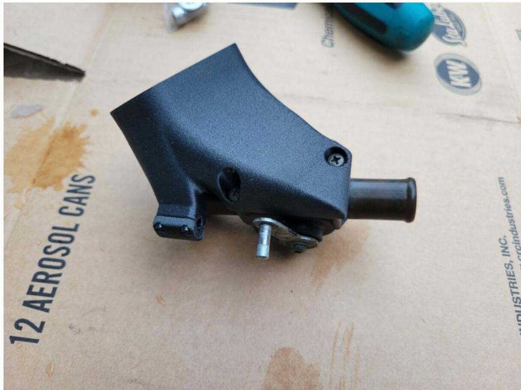
Install the new silicone hose onto the valve:
