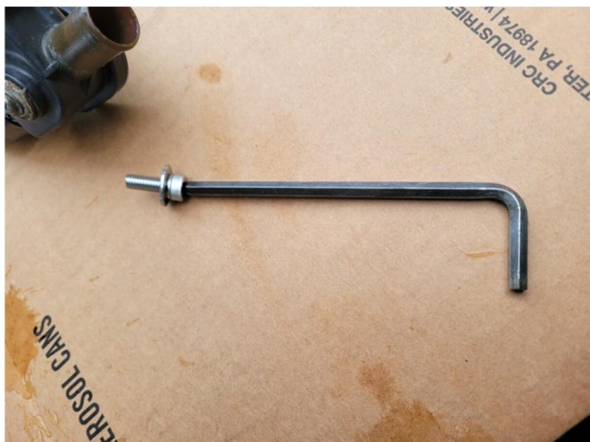
The clearance here is very tight. Put the bolts and washers into the holes on the bracket first then guide the silicone hose onto the heater core port as you place the valve roughly where it will live.
