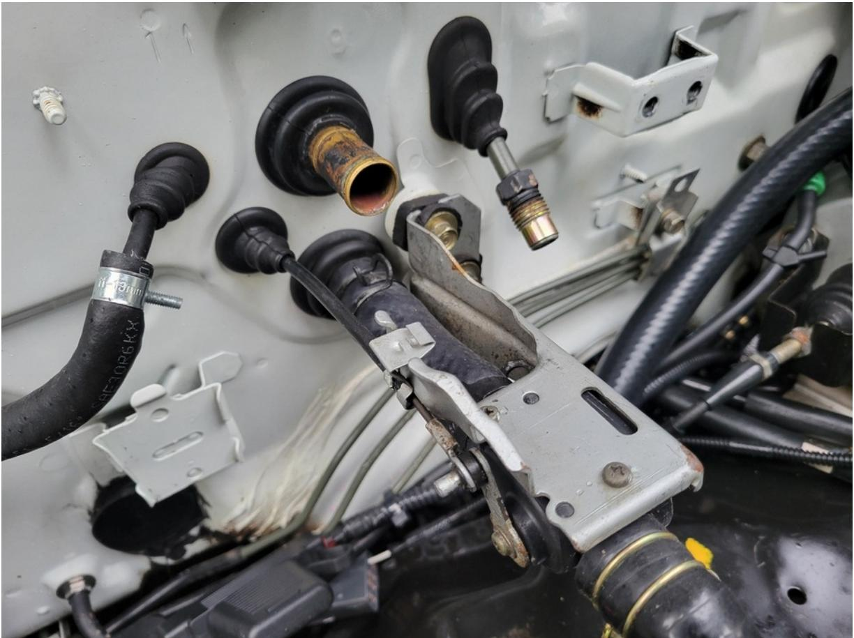
Unclip the control cable and remove it from the valve:
