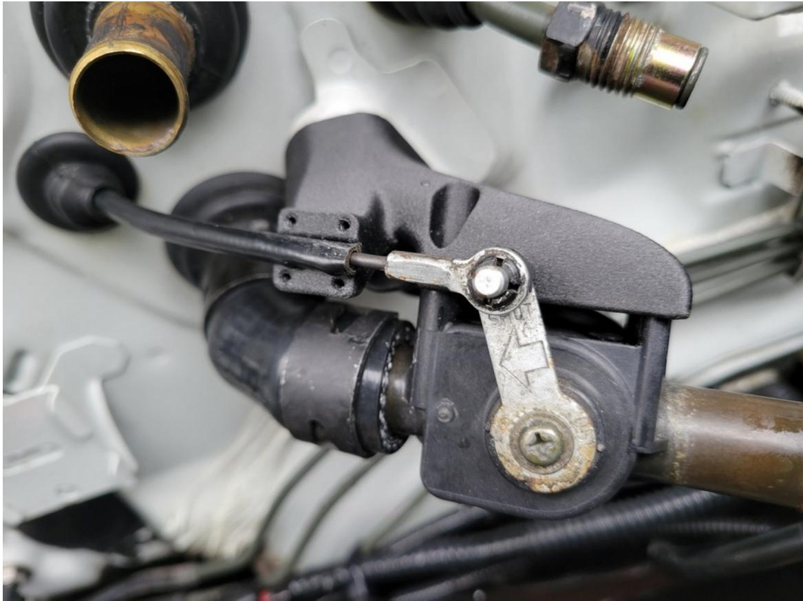
**Be careful not to over tighten the cable cap screws!** These are tiny screws that thread into plastic. Just run them down until they stop, then give it a very tiny extra twist.
