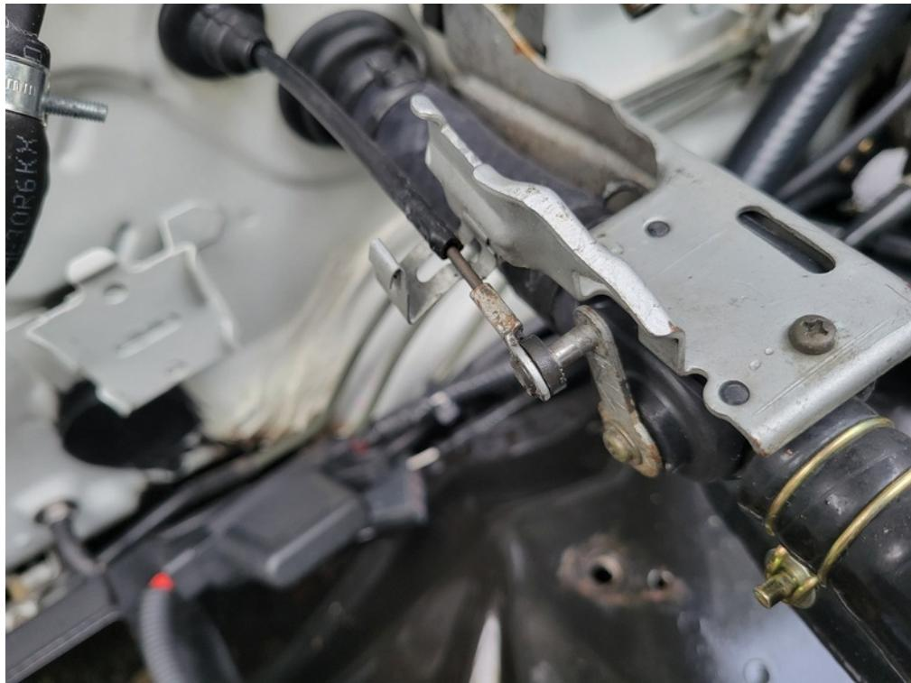
Remove the heater valve with the bracket and connector hose from the firewall:
