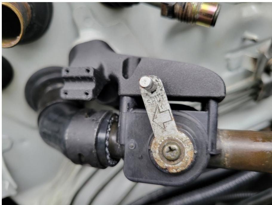
Place the control cable onto the valve. Make sure the valve is staying fully closed then install the cable cap again to secure the control cable:
