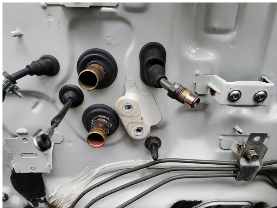
Take the heater valve off the stock bracket and keep the screws:
