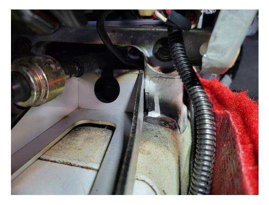
Use the body saw and/or die grinder to make clearance for the shifter base:
