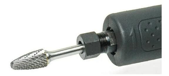
Use the die grinder with carbide burr to clean up the cuts. Test fit the base with shifter and remove any material needed until everything sits flat.
