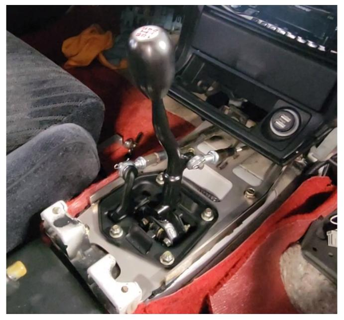
Now attach the cables to the shifter and the interior install is finished:
