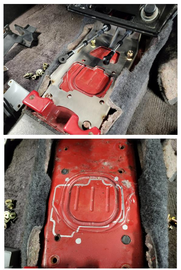
Snug the shifter base down then trace out the inner holes:
