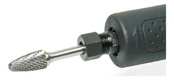
Use the die grinder with carbide burr to clean up the cuts. Test fit the base with shifter and remove any material needed until everything sits flat.
