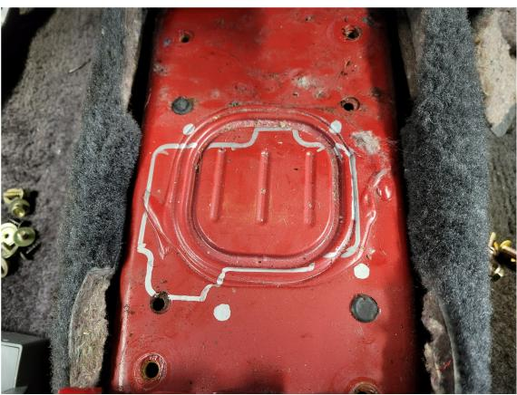
Use a small pilot drill bit to drill the center of the holes and inside of every corner. See the following image as an example:
