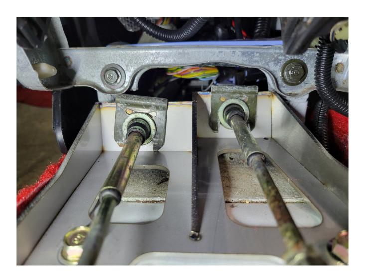
Now attach the cables to the shifter and the interior install is finished:
