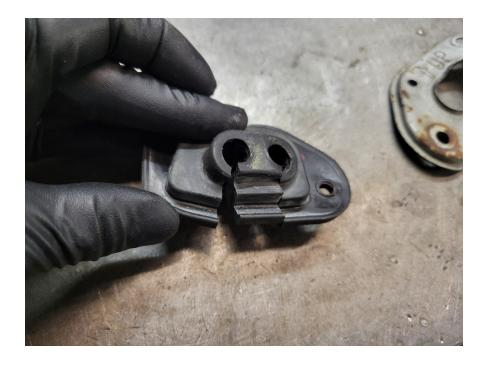
Install these parts onto the new cables in reverse order. We suggest coating the rubber grommet and cables here with some silicone spray during the install. It will make everything go together much easier:
