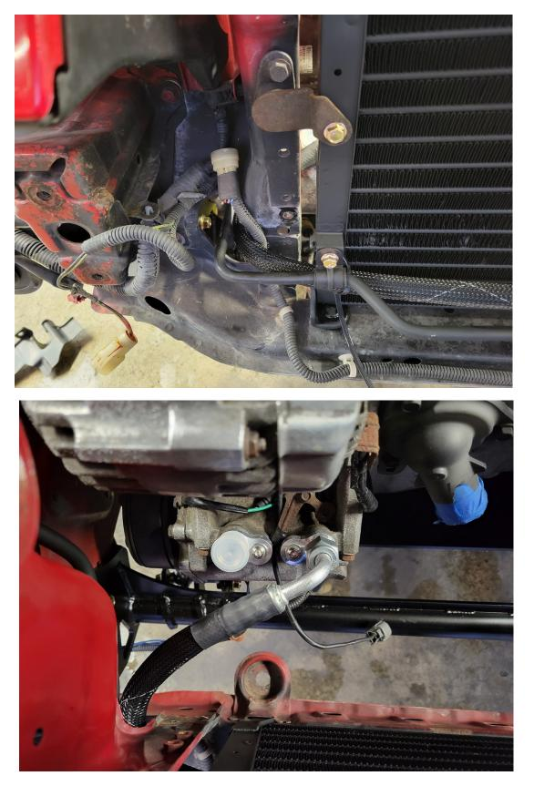
The suction and high-side lines can either run over or underneath the right side mount bracket. We will show going underneath in these instructions. Just skip further along if you are going over the bracket.
