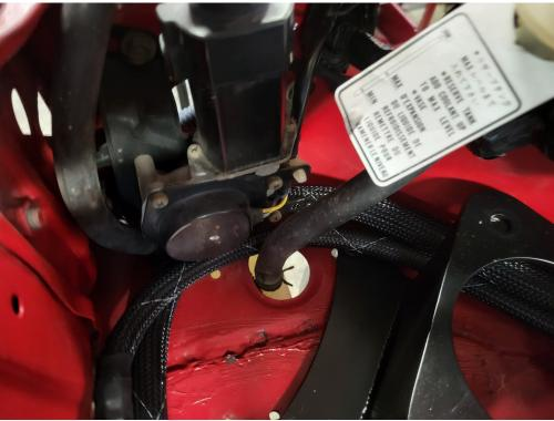
The lines should run around the coolant overflow hose like this:
