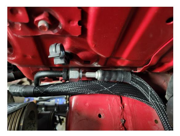
Connect the other ends of the suction and high-side lines to the evaporator fittings. This end of the line should run close to the chassis through the space between the brakes lines and chassis:
