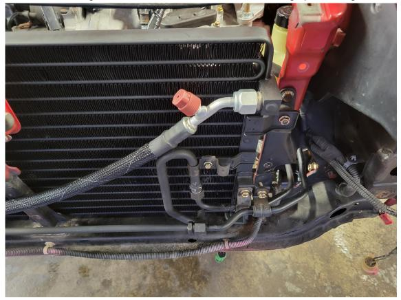
Route the other end of the discharge hose through the opening on the side of the condenser and then install it onto the compressor fitting:
