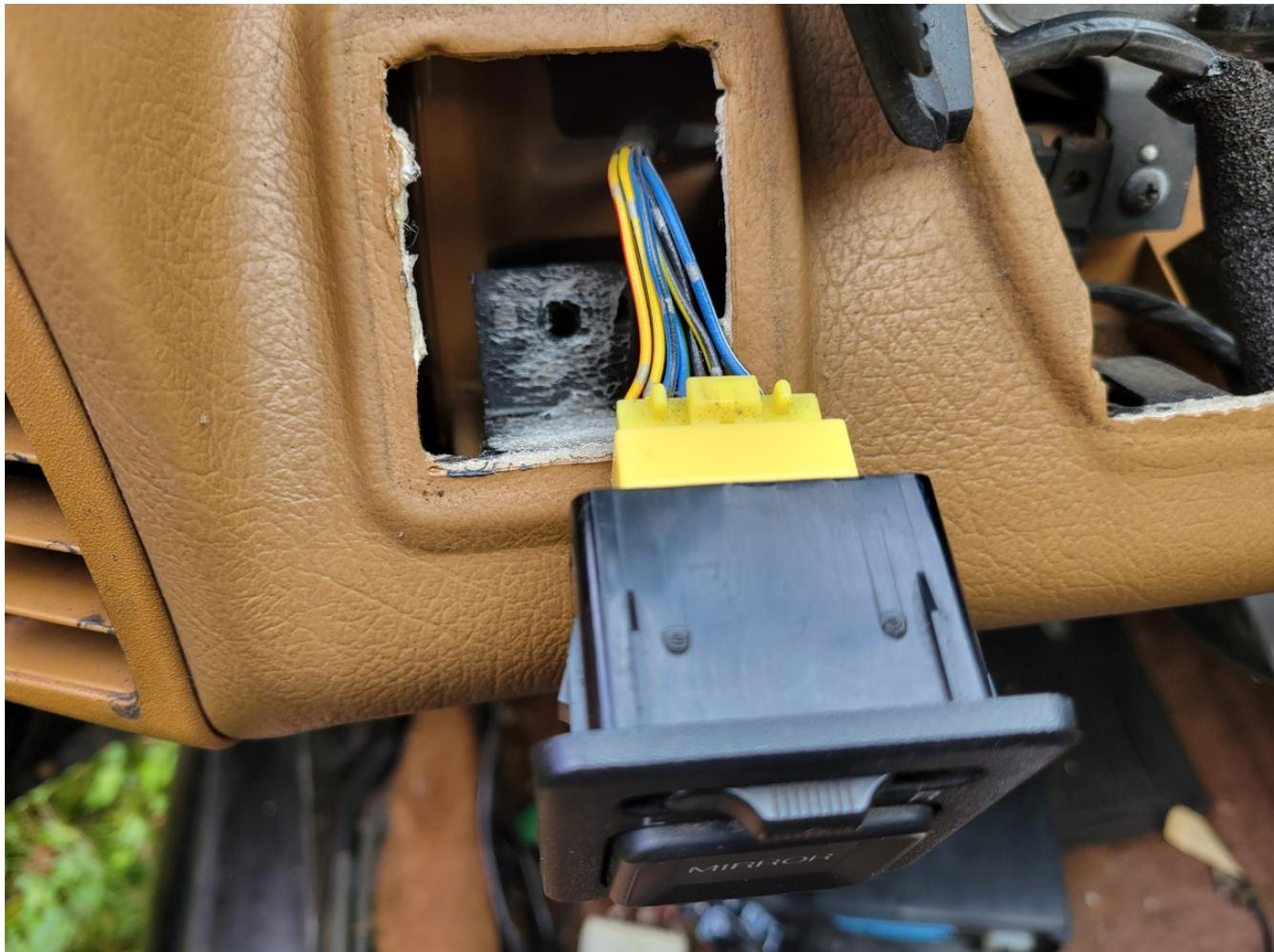
Push the new power mirror control delete into place then screw it in from below like before:
