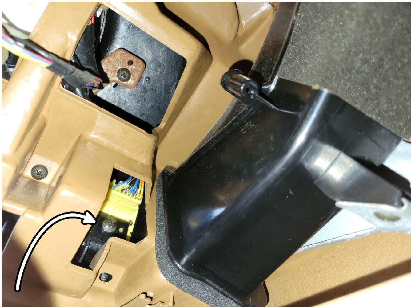
Pull the mirror control out of the front and disconnect the connector:
