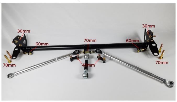
Here are the bolt length locations for the different block mounts:
