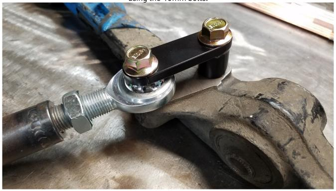
After that attach the front rod ends to the traction bar using the 60mm bolts.
