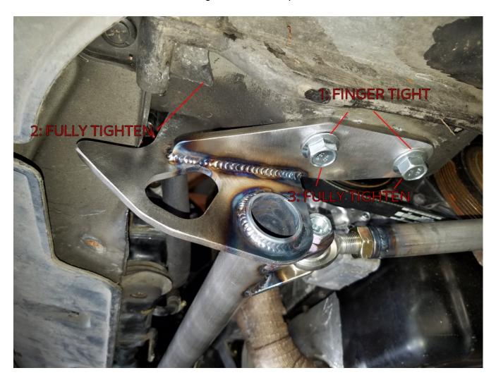
Put the control arm mounts into the radius rod rod ends and install both onto the control arms using the 40mm bolts:
