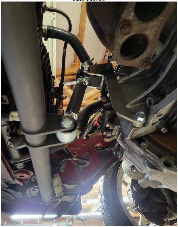
If you ordered the skid bar then it goes on by reusing the lower torque rod bolt as well as two additional 25mm bolts in the rear:
