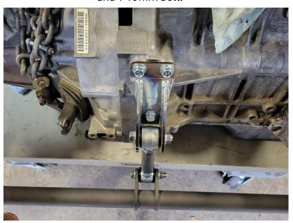
If you ordered the B series torque rod install the mount on the block. The 2 top bolts that go through the transmission bell housing are 70mm and the lower bolt that goes through the block is 80mm:
